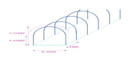
**Design of Walk-In-Tunnel**
